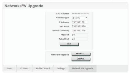
The Address Type dropdown allows selection between Static IP (manual configuration) or DHCP (automatic IP configuration) modes. When in STATIC mode the IP address, netmask and gateway can be defined manually. The HTTP and Telnet ports can also be changed from their defaults here. After making any changes, please press "Save" to store the new settings in the unit. If the IP address has been changed, it will be necessary to re-connect to the WebGUI using the new IP address.
