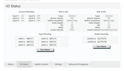
When a live input source is detected on one of the 6 HDMI inputs the corresponding input in this tab will display "ON". If no source is detected on that input, it will display "OFF".
