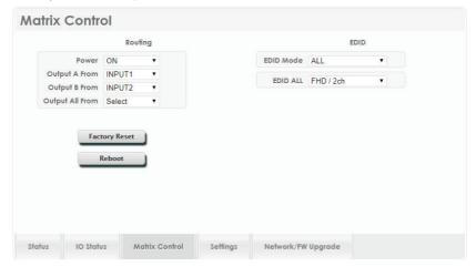
Any of the available inputs may be selected as a source for either of the two outputs by selecting the preferred input from the dropdown next to the "Output A" and "Output B" text.
