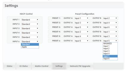
The HDCP mode for each input may be switched between the "Standard" and "Apple" modes. "Apple" mode allows for the display of non-HDCP required content from Apple, and similar, devices on non-HDCP displays.
