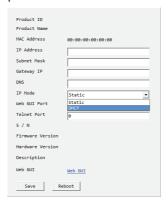
**IP Mode:** If you choose, you can alter the static IP network settings for the device, or switch the unit into DHCP mode to automatically obtain proper network settings from a local DHCP server. To switch to DHCP mode, please select DHCP from the IP mode drop-down, then click "Save" followed by "Reboot".
