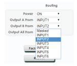
It is also possible to select a single source to be routed to both outputs quickly by selecting a source from the "Output All From" dropdown. Selecting "Masked" will output a blank video signal with no audio.
